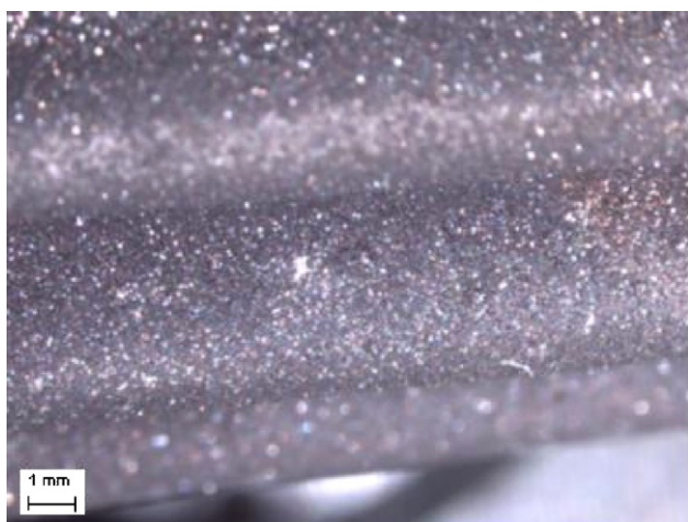
Fig. 6. Lateral view of a monolith with homogeneous washcoating.
